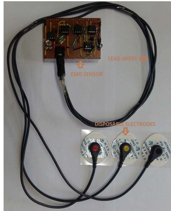
Fig. 6.1. Developed EMG sensor with electrodes and lead wires
